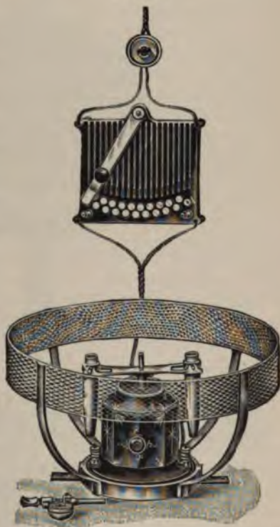
Improved electric hematocrit, with fender, rheostat, and speed-indicator. The hematocrit attachment replaces the urine tubes seen in the revolving armature.
